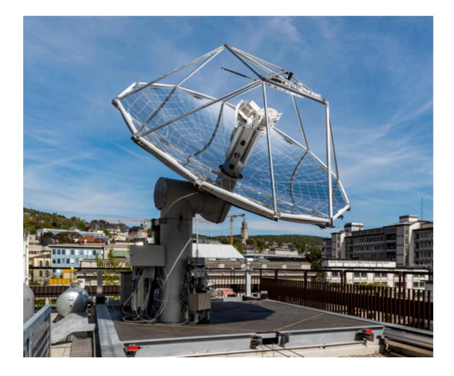
World first demonstration of complete thermochemical process for CO2-to-fuel with concentrating solar system (Aldo Steinfeld's group, June 2019, roof of ETH Zürich)
